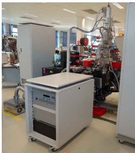
Rack for electronics & cooler
